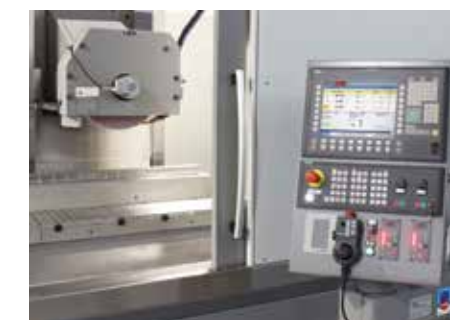
A Siemens CNC system installed on a MAXI 2000/750 grinding machine
